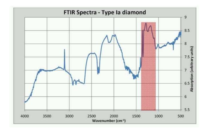
Note also that, although the absorption in the graphs above is in arbitrary units (and the background, as such, can be 'adjusted'), broadly speaking type IIa diamonds will have a lower IR absorption when compared to type Ia. Therefore, even if the region of research interest falls outside the nitrogen absorption range, it is recommended that one always uses type IIa diamonds when doing IR work.
